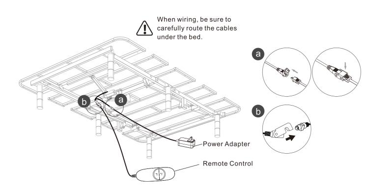
a. As shown in the diagram, after completing the connection, plug the power cord into a properly functioning power source. Use the remote control to raise the head and end of the bed to the highest angle. b. Place the bedspread on the bed frame first, then securely fasten the four straps at the head and end of the bed to their corresponding positions as shown in the diagram (the end with the metal buckles is for the end of the bed.
