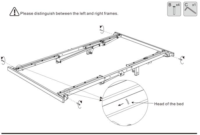
a. Paste the felt pads on the legs.(If already pasted, please ignore this step.) b. Lift the bed frame, install the bed legs, and tighten them.
