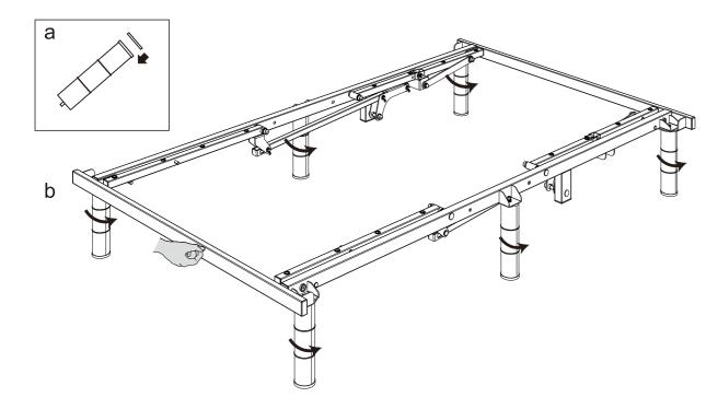
As shown in the diagram, please arrange the upper frame in the order of H1 to H5, ensuring that the sticker arrows are aligned with the direction of the lower frame.
