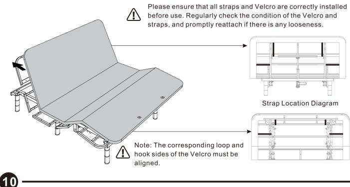
As shown in the diagram, use the remote control to adjust the bed to a flat position. Install the mattress retainer bar, then fasten the two straps on both sides of the middle bed frame to the corresponding positions shown in the diagram(The corresponding loop and hook sides of the Velcro must be aligned). Once all these steps are completed, the bed frame is ready for use.
