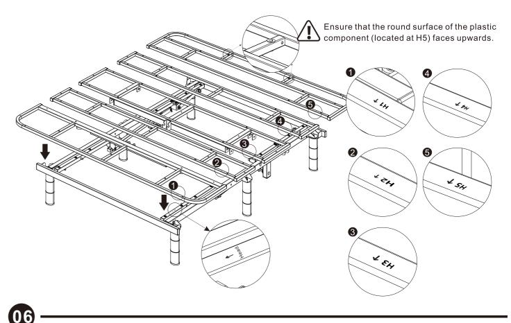
a. Please align the H1 with the protruding screw on the frame for installation. b. Please first loosely tighten the screws according to the diagram shown. Once all the screws are loosely tightened, fully tighten all the screws.
