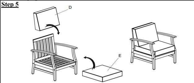
Inspect it and make sure all parts are adequately connected. Ensure all screws are fully locked into position and secured. Place Back Cushion (D) and Seat Cushion (E) on to the Chair
