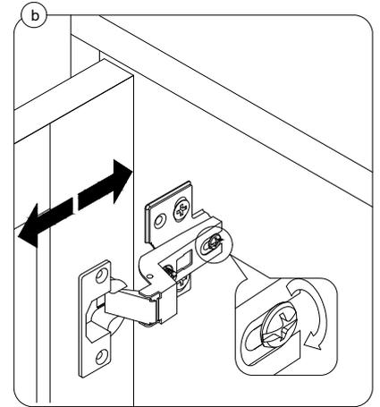
EN:To adjust the door laterally adjust the screw as shown byturning clockwise or anti-clockwise.
