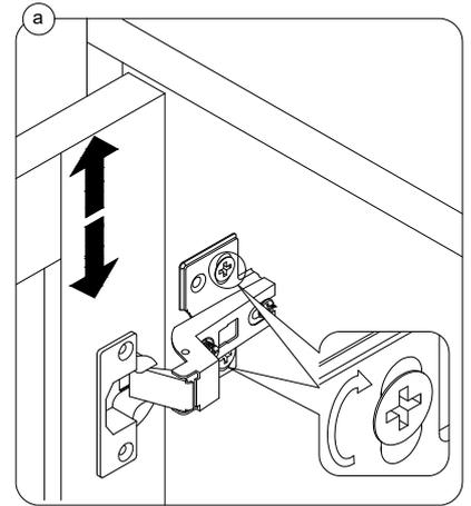
EN:To adjust the gap from the door to the main frame turn thescrew clockwise or anti-clockwise as needed.
