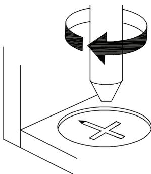
**EN\_**Turn cam lock clockwise to tighten.
