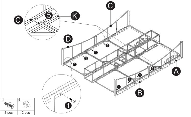
STEP 10 Connect step 9, part (L), (M), (N), (O) and using bolt (1)
