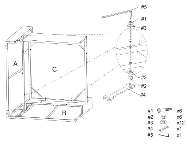
Step 3. Attach arm panel (part A) to assembled unit (parts C&B) using bolts (part #1), washers (part #3), nuts (part #2), wrench (part #4) and allen key (part #5).
