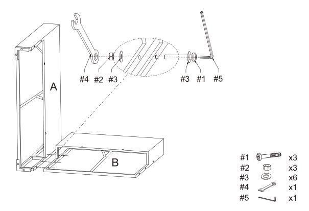
Step 2. Attach seat panel (part C) to assembled unit (parts A&B) using bolts (part #1), washers (part #3), nuts (part #2), wrench (part #4) and allen key (part #5).
