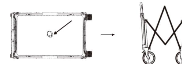
3. When not in use, press and hold the middle button on the pull rod to shorten the pull rod. When in use, directly pull out the pull rod. The pull rod can be positioned within 90 degrees and can be subjected to forces used by people of different heights.
