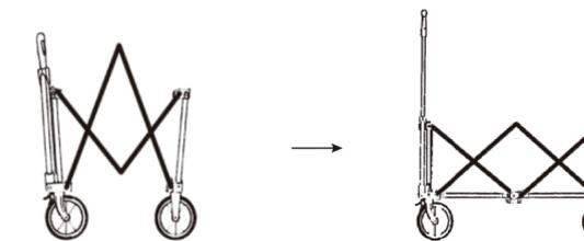
**2. Folding and storing:** After taking out the folding bottom plate, gently lift the bottom center pull ring, and the frame will automatically collapse.
