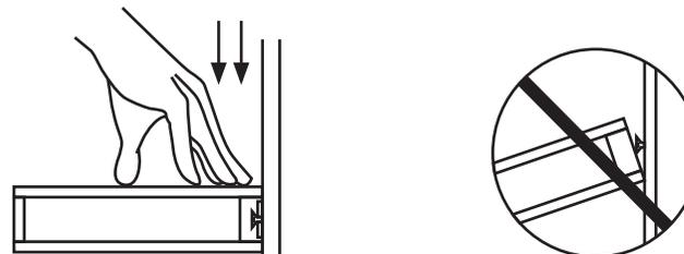
If shelf cannot hang on to the screws, untighten the screws slightly and re-hang. Repeat as necessary.
