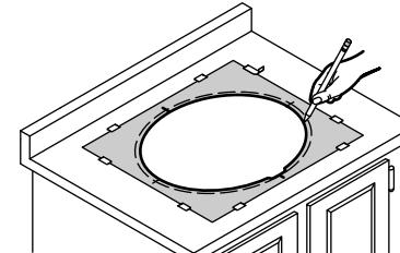
**3 Drill a pilot hole and cut the countertop opening along the inside line.**
