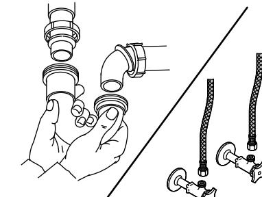
**7 Apply sealant and wipe away any excess. Fill voids and allow to dry.**
