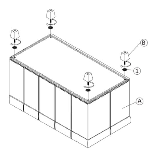
Place Ottoman (A) on its back on a flat smooth surface. Attach Feet (B) with Washers (1) to each corner.
