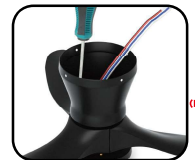
6 Rotate the controller cover to position 2 screw holes of each blade in turn and tighten blades with screws.
