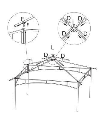
Step 3:Insert the small head of Part F to the long side of Part D directly and insert one Part K to the other head of Part F.
