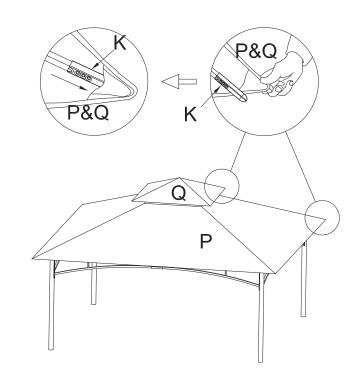
Step 6:Put the canopy fabric (Part P&Q) on the frame, extend it fully. Put the heads of tubes(Part K) into the corner pocket of canopy fabric.
