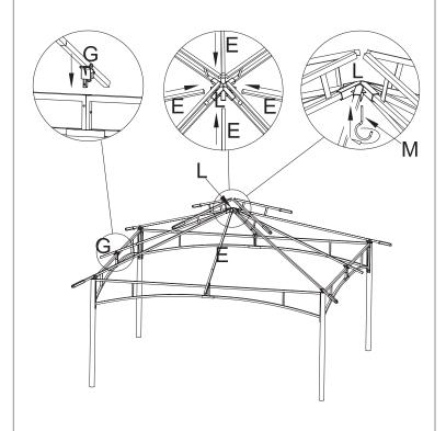
Step 5:Insert Part G to the middle part of the two attached part C. The other three Part G should be done as this. Then insert the other head of Part E to Part L. Finally, Insert Part M(the steel hook) to the hole of Part L and turn it to tighten it.
