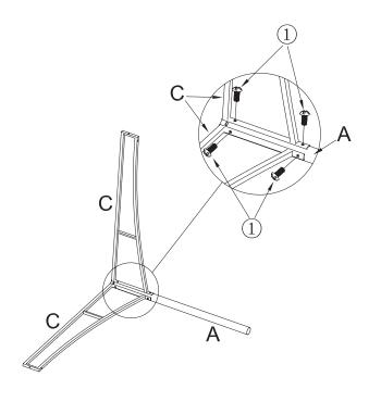
Step 1:Put two Part C together and put one Part A in the middle of them,then use Screw① to tighten Part C and Part A.
