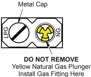
**Use only the cap supplied on the regulator. Do not use an off the shelf pipe plug. This can damage the plunger. The supplied regulator cap is designed so it will not engage the unused gas type.**
