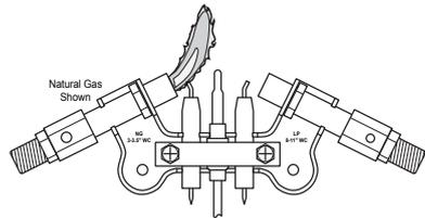
**Figure 30 - Incorrect Pilot Flame Pattern (Natural Gas shown)**
