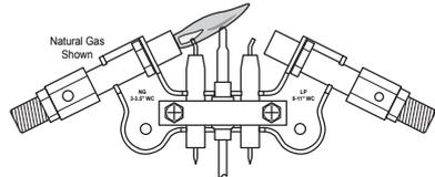
**Figure 29 - Correct Pilot Flame Pattern (Natural Gas shown)**
