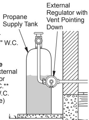
**Figure 14 - External Regulator with Vent Pointing Down**
