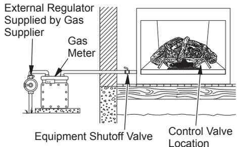
**Figure 17 - Checking Gas Joints for Natural Gas**
