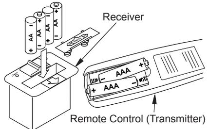
**Figure 19 - Installing Batteries in Remote Control and Receiver**
