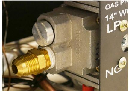
**Use only the metal cap. DO NOT use an off the shelf 3/8" NPT pipe plug. This will damage the plungers located inside the regulator.**
