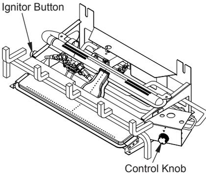
**Figure 22 - Ignitor Button and Control Knob Locations**
