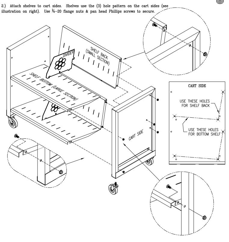
3.) After cart sides and shelves are assembled, turn unit upside down and insert (4) casters into sockets on bottom of cart.
