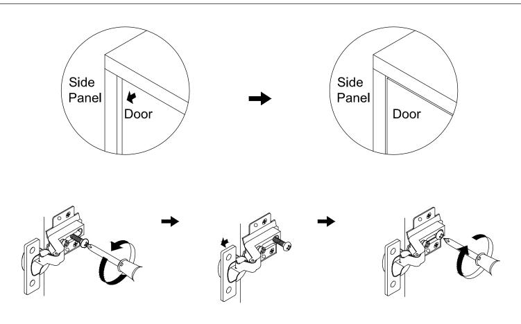
If the top of the door is not level with the side panel, loosen the screw at the back of the hinge as shown, then move the hinge in or out until the desired gap is achieved, and then re-tighten the back screw as shown.
