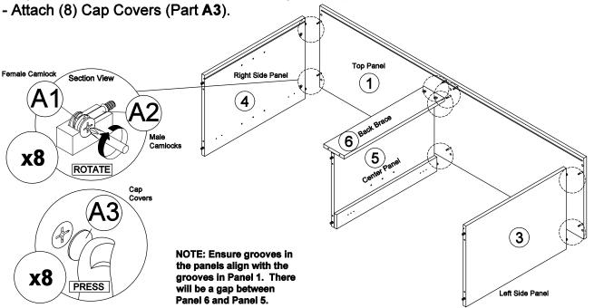
\* In this step Female Camlock A1, Male Camlock A2 and Wood Dowels B are pre-inserted.
