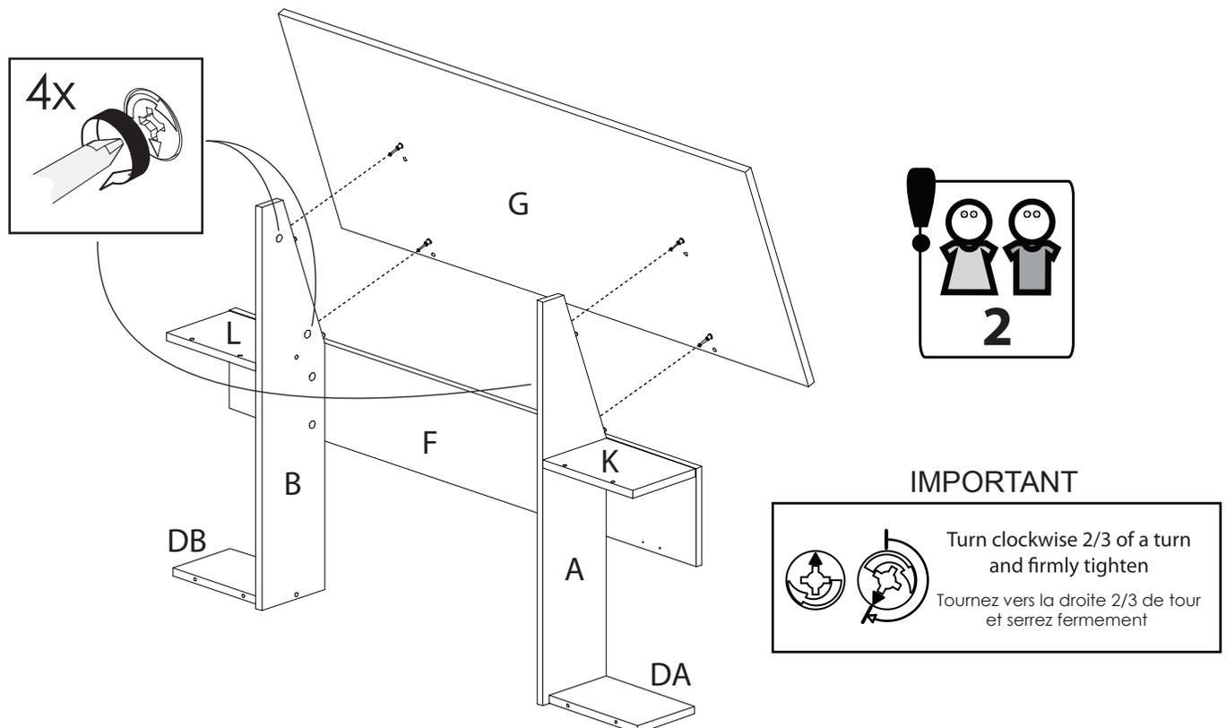
**8** Use the Allen key # 2300 and 6 screws # 0111 to secure your headboard to the bed frame.
