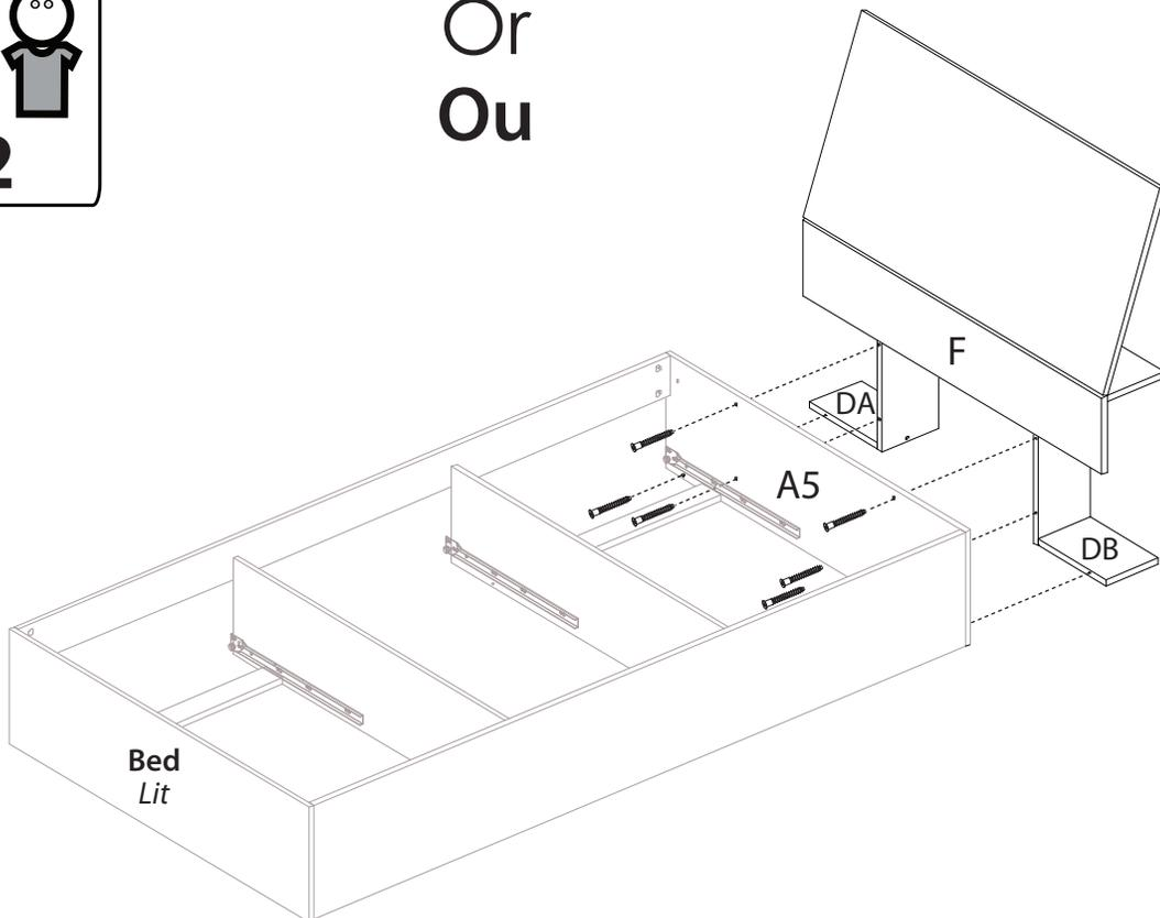
**9** Use the 8 screws # 0120 to fasten the 2 metal plates # 0602 to the panel F of the headboard and the panel A5 of the bed frame. Refer to the pilot holes drilled on the panel F to set the location of the 2 metal plates
