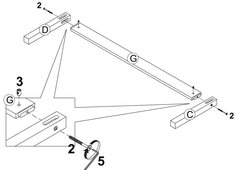
**Note:** Part 3 will face up with the "x" mark on it, otherwise it cannot be tightened.
