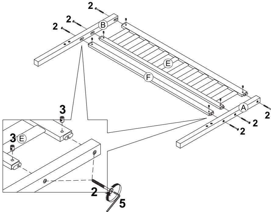
**Note:** Part 3 will face up with the "x" mark on it, otherwise it cannot be tightened.
