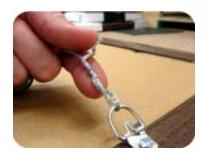
Step 5: Twist the wire around itself several times, as shown. To ensure secure hanging, loop a portion of the wire back through itself. Use caution when handling the wire so as not to poke yourself on the wire ends.
