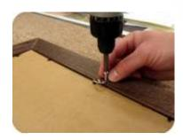
Step 3: The D-rings should be installed using the screws provided. An electric / battery powered screw driver or drill is strongly suggested. The D-rings should be installed so the flat portion is on the frame and the ring is hanging over the backing of the frame. This step is repeated for both the left and right sides of the frame. DO NOT attempt to install D-rings on the cardboard backing of the frame.
