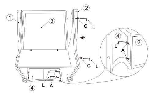
Step 3:Secure right arm (2) to assembled chair back (3) with 2 screws (C) by using allen wrench(L). Then, secure seat panel (4) to assembled right arm (2) with 2 screws (A) by using allen wrench (L). Please tighten all screws now.
