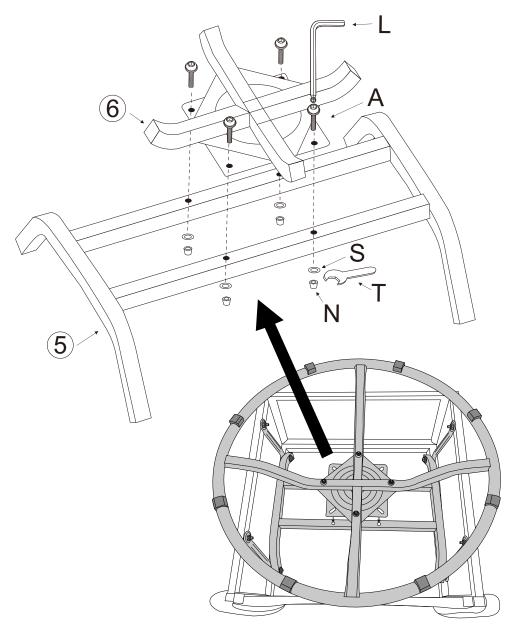
Step 5: Rotate the top plate on the chair base (6) into correct position, make sure it matches the holes on the swing bracket. Connect the 4 screws (A) through the holes of the plate on the base (6) and the holes on the tube of swing bracket (5) with 4 flat washers (S) and 4 nuts (N) by using allen washer (L) and open end wrench (T). NOTE: THIS STEP IS VERY IMPORTANT. DO READ THE INSTRUCTION AND DIAGRAM CAREFULLY.
