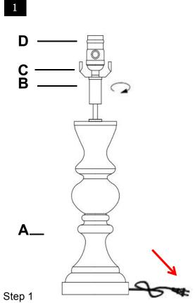
Pull power cord to connect the Neck (B) to the Base (A). Screw the Neck (B) onto the Lamp base (A) Be careful not to twist the power cord and tighten securely
