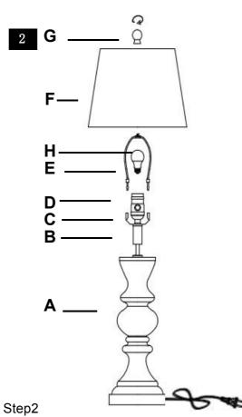
Insert the Harp (E) into the Saddle (C). Put the shade(F) on the Harp(E),then tighten the Finial (G)into the Harp (E) Insert the bulb(H) into the socket(D).
