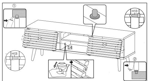
**STEP9**: Hold the frame door with position of the upper pin shown facing upward. Put the frame door by inserting it to the upper groove on Top Board (A), then place the lower part aligned into the groove on bottom board (B). Repeat this step for the other door. Slide the item's doors left and right to ensure the doors have been placed properly on the track.
