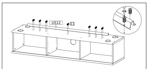
**STEP5**: Place Anti Deflection Metal Bar (HW US12), secure with screw M6x12.5 mm (HW11) using screwdriver.
