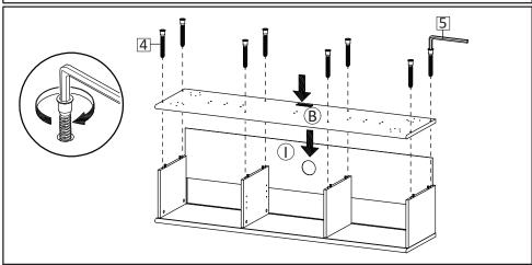
**Step3**: Insert Backboard (I) as shown in the figure above. Place bottom board on top and secure with Screw M7x50 mm (HW4), tighten screws using Allen Key (HW5).
