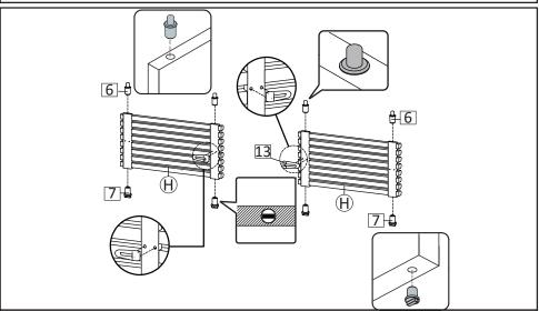
**STEP8**: Insert Stopper (HW13), position as shown in the figure. Insert Top Pin Sliding (HW6) and Bottom Pin Sliding (HW7) on both end of frame door as specified position in the figure.
