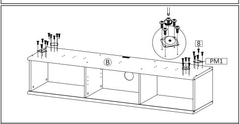
**Step4**: Install Mounting Plate (HW PM1) and secure with Screw M4.5x12.5 mm (HW8) into Bottom Board (B).
