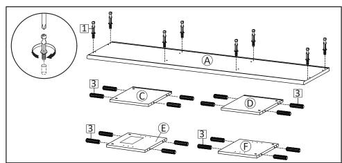
**STEP1**: Insert Cambolt (HW1) into Top Board (A). Insert Dowel (HW3) into Center Boards (E&F), Side Board Left (C) and Side Board Right (D).
