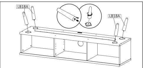
**STEP6**: Insert Leg (LB18A) into Mounting Plate, tighten by rotating . the leg clockwise.
