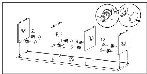
**STEP2**: Attach Side Board Left (C), Side Board Right (D), Center Boards (E&F) to Top Board (A). Insert Camlock (HW2) then tighten using screwdriver. Put Screw Cap (HW12) over the camlock.
