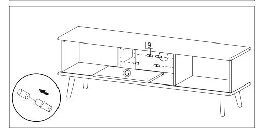
**STEP7**: Insert Shelf Pin (HW9) into the provided holes on both Center Boards at the desired level. Then place the Adjustable Shelf (G) onto the Shelf Pin.
