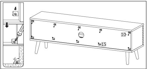
**STEP10**: Using Wedge (HW15) and Screw M3.5x15.5 mm (HW10) tighten the back of media stand with screwdriver.
