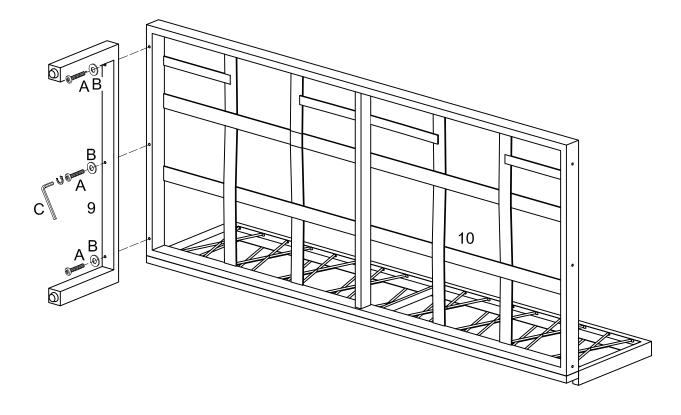
Use wrench (C), bolt (A), washer (B) to secure the leg (9) to the seat frame (10).
