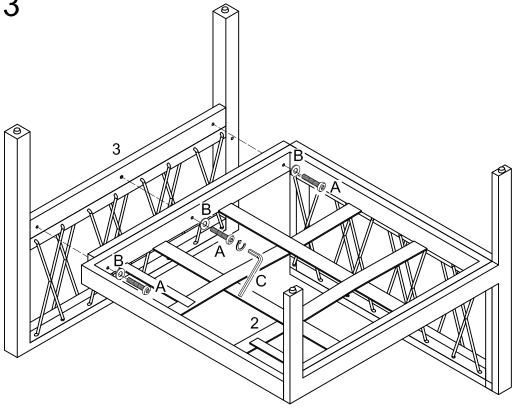
Use wrench (C), bolt (A), washer (B) to secure the seat frame (2) to the side frame (3).
