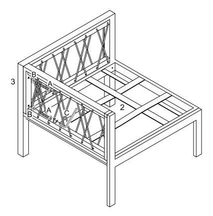
Use wrench (C), bolt (A), washer (B) to secure the back frame (4) to the side frame (3).
