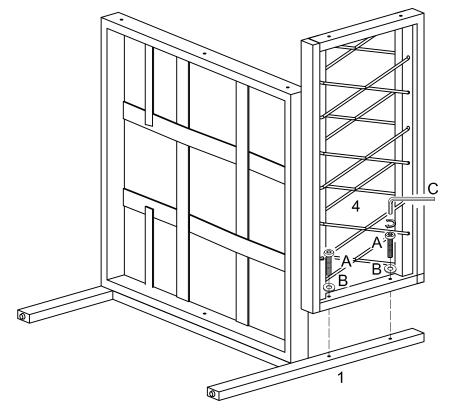
Use wrench (C), bolt (A), washer (B) to secure the back frame (4) to the side frame (1).
