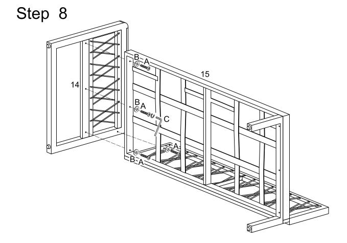
Use wrench (C), bolt (A), washer (B) to secure the seat frame (15) to the side frame (14).
