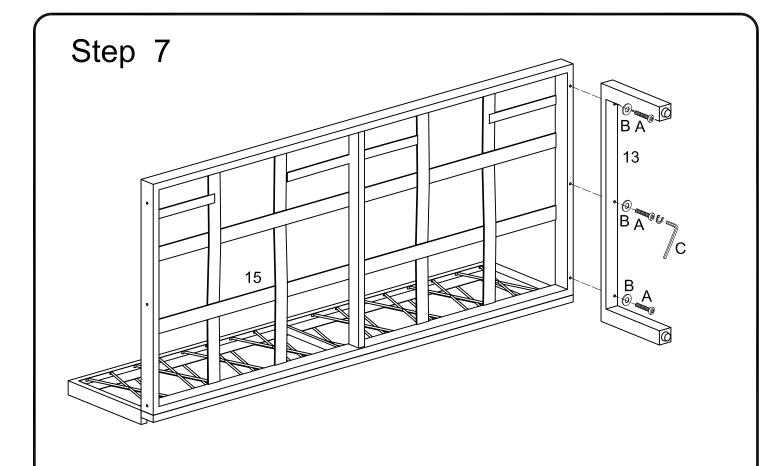
Use wrench (C), bolt (A), washer (B) to secure the leg (13) to the seat frame (15).
