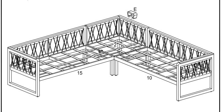
Place the U shape buckle (E) to connect with the seat frame(2,10)
