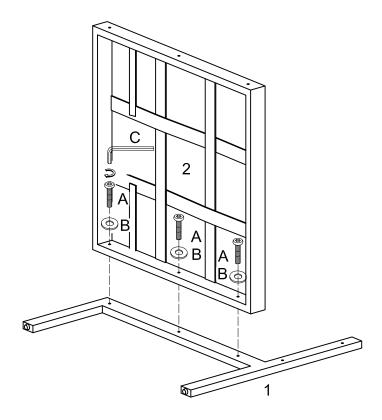
Use wrench (C), bolt (A), washer (B) to secure the seat frame (2) to the side frame (1).
