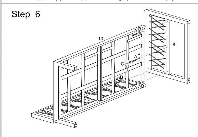
Use wrench (C), bolt (A), washer (B) to secure the seat frame (10) to the side frame (8).
