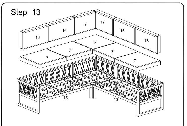
Place the cushion (5,6,7,16,17) on top of the seat frame (15,2,10) as per diagram.
