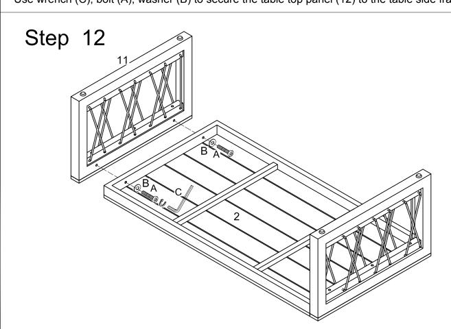
Use wrench (C), bolt (A), washer (B) to secure the table top panel (12) to the table side frame (11).
