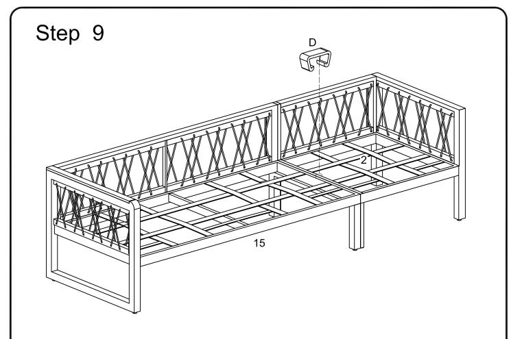
Place the (big) U shape buckle (D) to connect with the seat frame(15,2)
