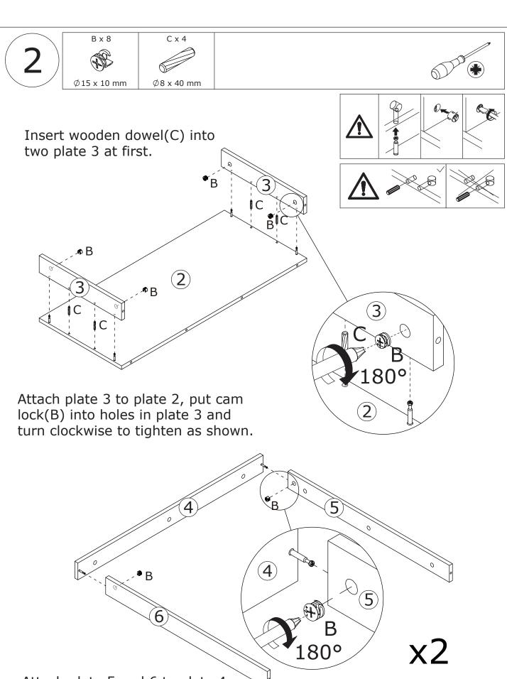
Attach plate 5 and 6 to plate 4, put cam lock(B) into holes in plate 5, 6 and turn clockwise to tighten as shown.
