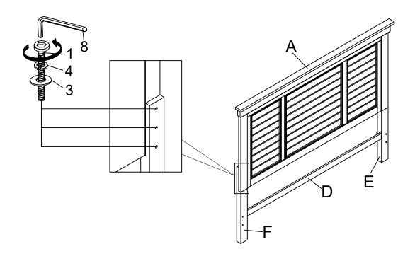
STEP 2 Assemble the HB crossbar (D) to HB legs (E & F) by using Allen Key (8)with hardware 1,3, and 4. \*TIGHTEN ALL THE BOLTS BY USING ALLEN KEY (8)
