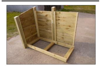
Remove the blocks from beneath the 2nd panel and then slide the base into position as shown, ensuring that the centre post and the central cross member of the base are aligned centrally.
