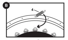
Swing the **SPRING 4** to face inside of the trampoline. Refer to illustration B.
