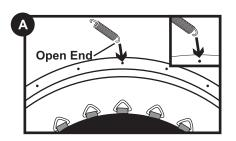
Find the open end of the **SPRING** 4 and hook this end into the hole on the **RAIL(1,2,3,4).** Refer to illustration A.
