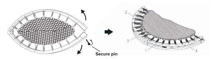
**Note:** Check that all the springs are attached before continuing to assemble the trampoline. If any spring is not attached or damaged Then follow this process -
