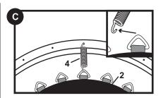
Slide the metal loop on the **MAT** ② into the spring hook as shown in illustration C.
