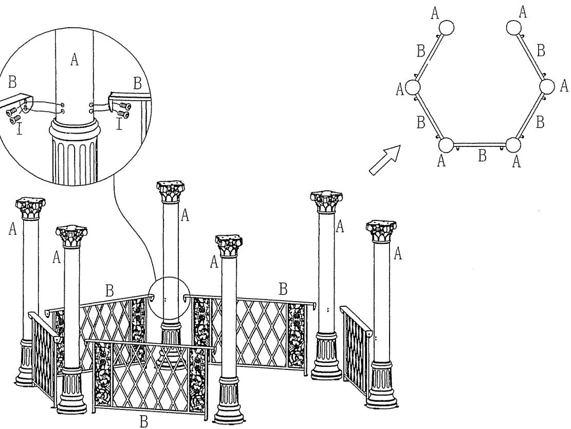
2 Put small poles onto the top of big poles, Assemble it with bolt(I).
