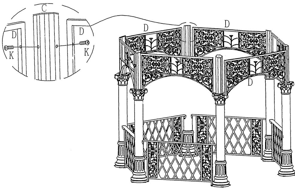
4 Insert girder into top connection pont, then attach girder to small poles wiht bolt(J) as the picture, tighten all bolts.
