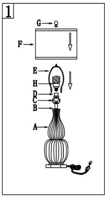
Step 1 Make sure all parts could be aligned before assemble Insert the harp (E) into the saddle (C). Put the shade(F) on the harp(E),then
