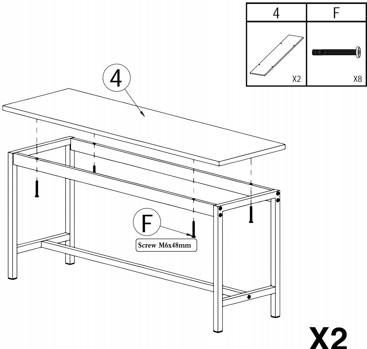
EN-During the assembly, please first half-tighten all the screws into the holes.
