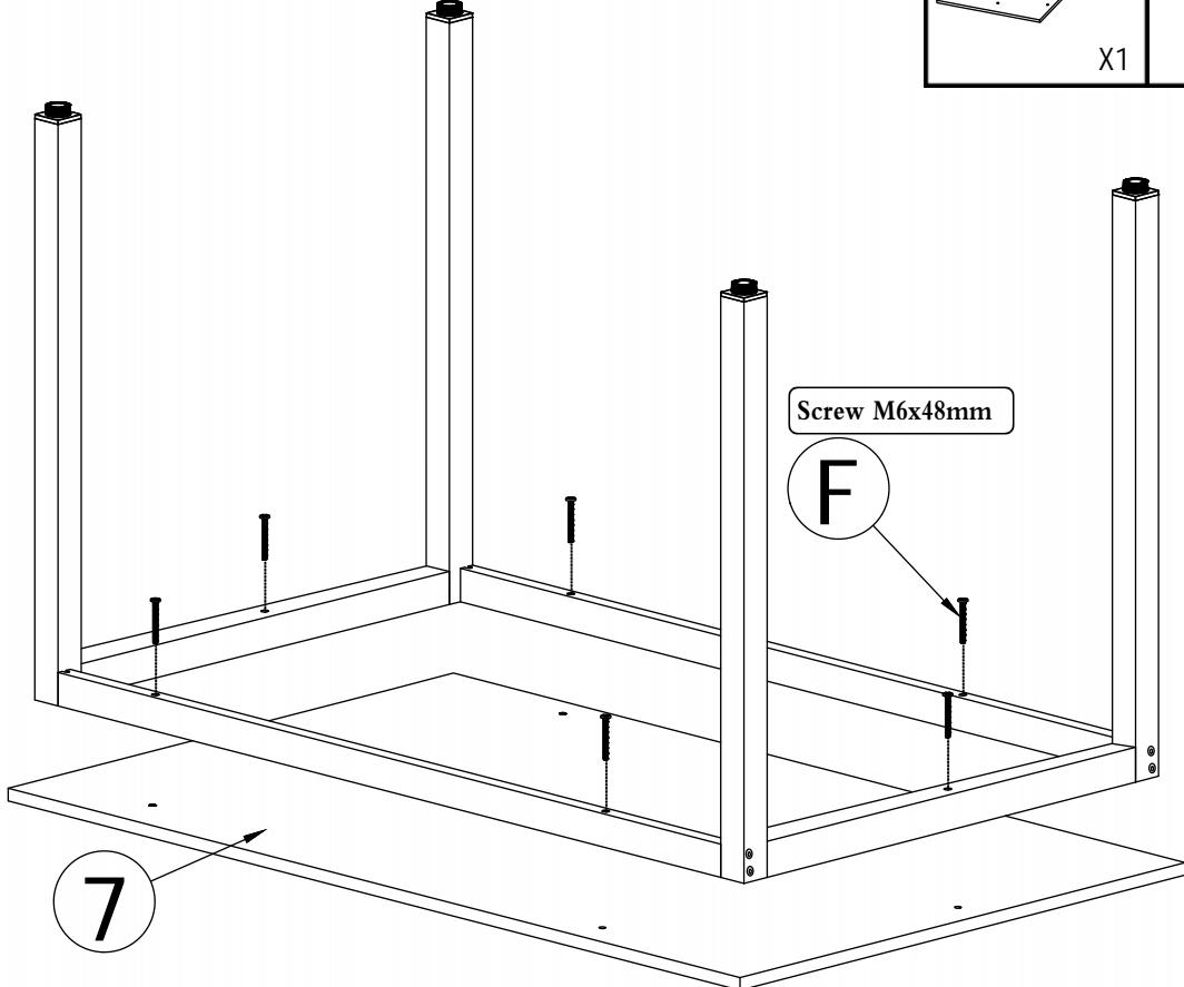
EN-During the assembly, please first half-tighten all the screws into the holes.
