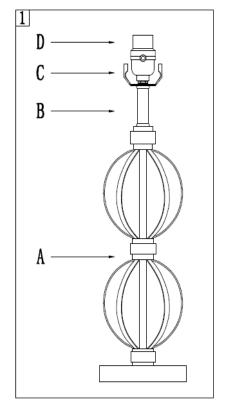
Step 1 Screw the Neck (B) onto the Lamp base (A) Be careful not to twist the power cord and tighten securely
