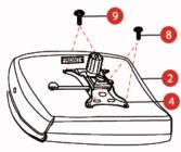
Align the Seat Plate(4) over the pre-drilled holes underneath the Seat Cushion(2), make sure that the front of the Seat Plate is facing the front of the Seat Cushion. Attach the Seat Plate to the Seat Cushion using Two Bolts M8\*30mm(9) at the front and Two Bolts M8\*25mm(8) at the back, tighten all the bolts with the Wrench(13), being careful not to miss-thread the bolts or damaged the Seat.
