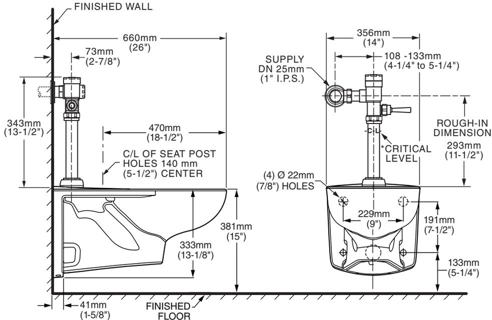
\*Note: The Critical Line (-C-L-) on Vacuum Breaker must typically be a minimum of 6" (152mm) above fixture. Consult Codes for details.
