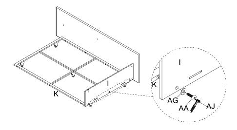
Insert the Drawer Bottom Board (L) to the Drawer Side Board (I).
