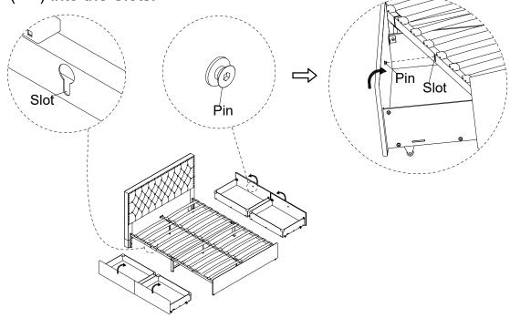
When pull out the drawers, lift the drawers first in order to make the Pins released from the Slots freely, then pull the drawers toward outside. DO NOT PULL OUT THE DRAWERS DIRECTLY.
