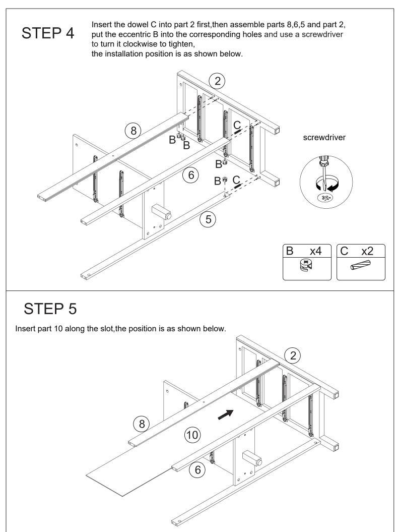
Insert the dowel C into part 3 first, then assemble parts 8,6,5 and part 3, put the eccentric B into the corresponding holes and use a screwdriver to turn it clockwise to tighten, the installation position is as shown below.
