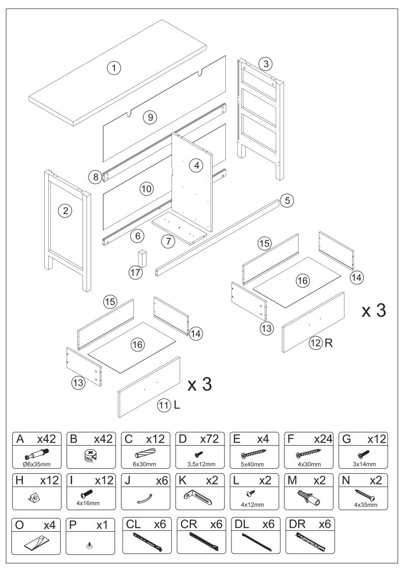
First Lock the guide rail CL to the right side of the part 4 with screw D, then turn it 180 degrees and lock the guide rail CR to the left side of the part 4 with the screw D, the installation position is as shown below.
