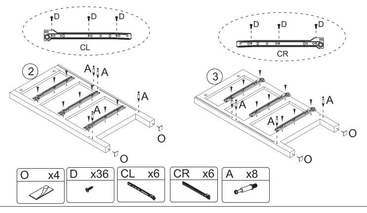
Install the screw A on the part 6,5
