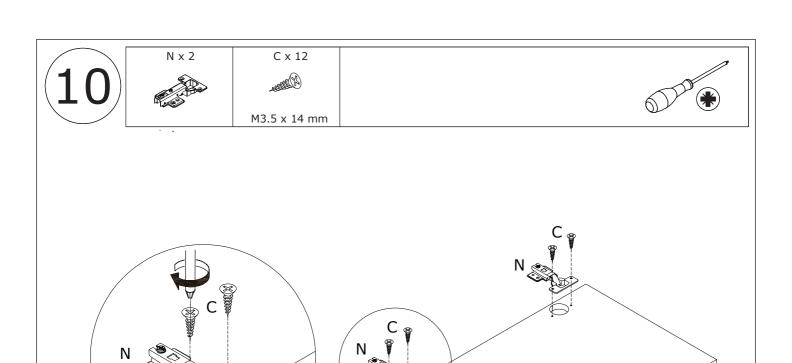
Fix hinge(N) to board 10 with screw(C) as shown. Attach door 10 to board 8 by fixing hinge with screw(C) as shown.
