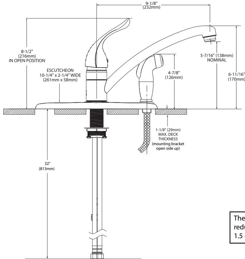
The use of aerator part 116711 reduces flow to a maximum of 1.5 gpm (5.7L/min.)
