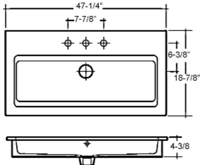
Dimensions of fixture are nominal and may vary within the range of tolerances established by ASME Standard A112.19.2-2008. Dimensions and specifications subject to change without notice.
