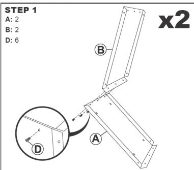
Align the lip of one Solid Panel (B) with the inside of one Expansion Panel (A) and loosely secure using three M6x10mm Bolts (D).
