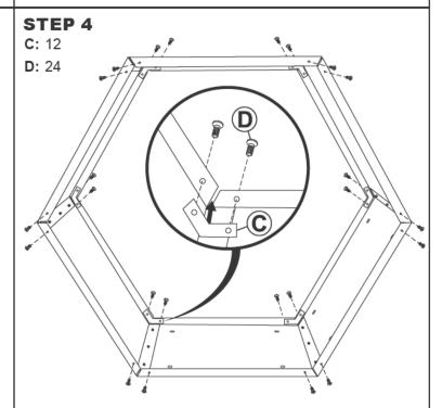
Loosely secure one Bracket (C) onto each inside corner using two M6x10mm Bolts (D).
