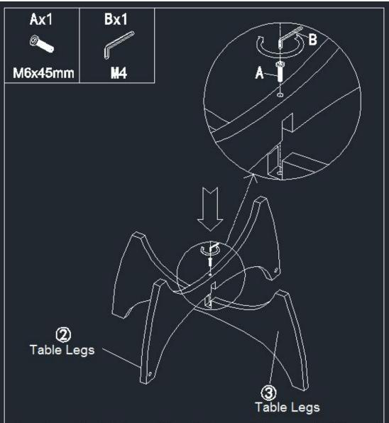
Step 1, put ② table leg on ③ table leg, use "A" part to fix it from the bottom hole of ③ table leg, and use "B" part to tighten "A" screw. NOTE:
