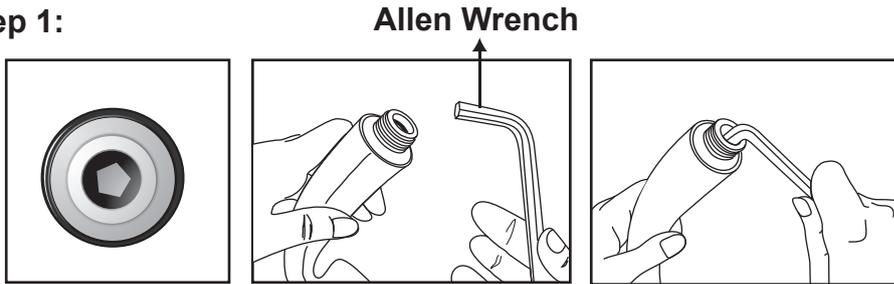
Insert the Allen Wrench Into the bottom of the handheld shower.
