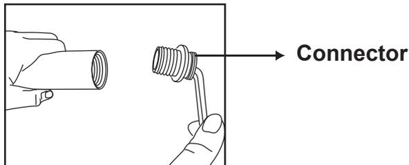
Remove the Connector by turning the Allen Wrench counter-clockwise.
