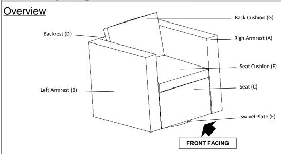
This Swivel Chair has multiple parts and may require up to 30 minutes to assemble. To give you an overview of the Swivel Chair parts, the above picture is to help you put the various parts into perspective. Please read through the instructions below to familiarise yourself with the parts and steps before assembly.
