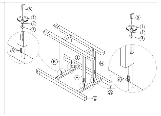
Assemble the part in step (4), into the part in step (2), using the wooden dowel (6), bolt (1), Spring Washer (4) flat washer (5), Allen key (8). **Do not fully tighten Bolts at this time.**
