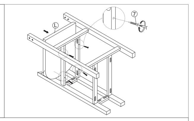
Assemble the Seat Frame With Cushion (L), into the part in step (5), using the Wood screws (7). Do not fully tighten Bolts at this time.
