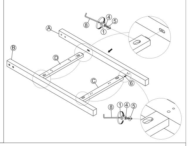
Assemble the Stretcher lower front leg (C), Stretcher the upper front leg (D) into the Left front leg (A), Right front leg (B), using the wooden dowel (6), bolt (1), Spring Washer (4) flat washer (5), Allen key (8). **Do not fully tighten Bolts at this time.**
