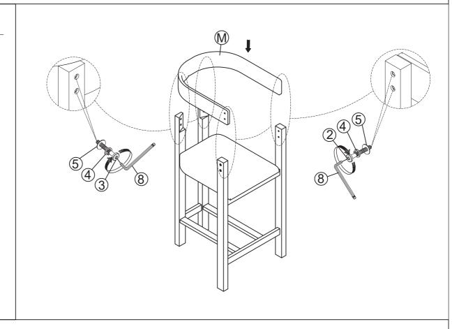
Assemble the Back Frame (M), into the part in step (6), using the bolt (2) for the front and (3), for the back , Spring Washer (4) flat washer (5), Allen key (8).
