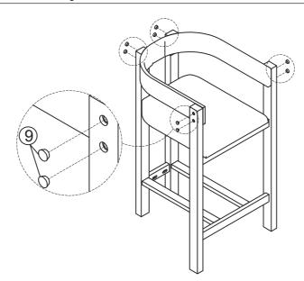
Close the Wooden Plugs (9) tightly to the previous bolt catch hole.
