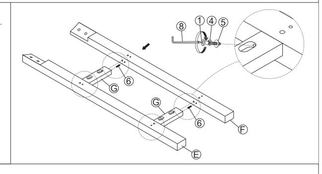
Assemble the Stretcher the back leg (G),into the Left back leg (E),Right back leg (F),using the wooden dowel (6), bolt (1), Spring Washer (4) flat washer (5), Allen key (8). **Do not fully tighten Bolts at this time.**
