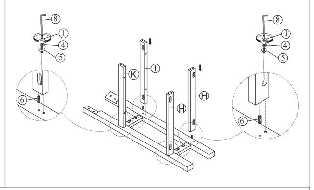
Assemble the Lower middle leg stretcher (H), Right Upper middle leg stretcher (I) Left Upper middle leg stretcher (K), into the part in step (3), using the wooden dowel (6), bolt (1), Spring Washer (4) flat washer (5), Allen key (8). **Do not fully tighten Bolts at this time.**
