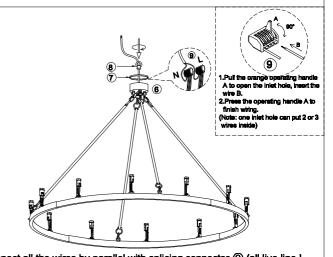
3.Connect all the wires by parallel with splicing connector (all live line-L use one connector, and neutral Line-N use another connector).
