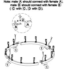
1.Assembled the split parts ① to a completely ring fixture like picture showed, pushed the split parts and fix with bolt screw ②.
