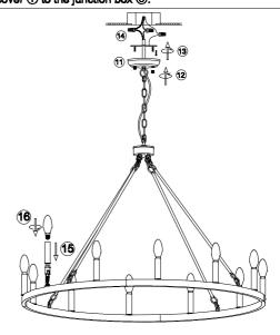
6.Install the bracket to the ceiling junction box with screw (3).
