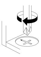
Turn cam lock clockwise to tighten.
