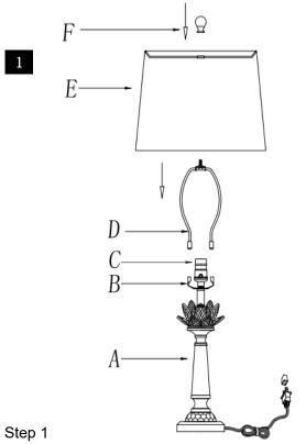
Insert the Harp (D) into the Saddle (B). Put the shade(E) on the Harp(D), then tighten the Finial (F)into the Harp (D)
