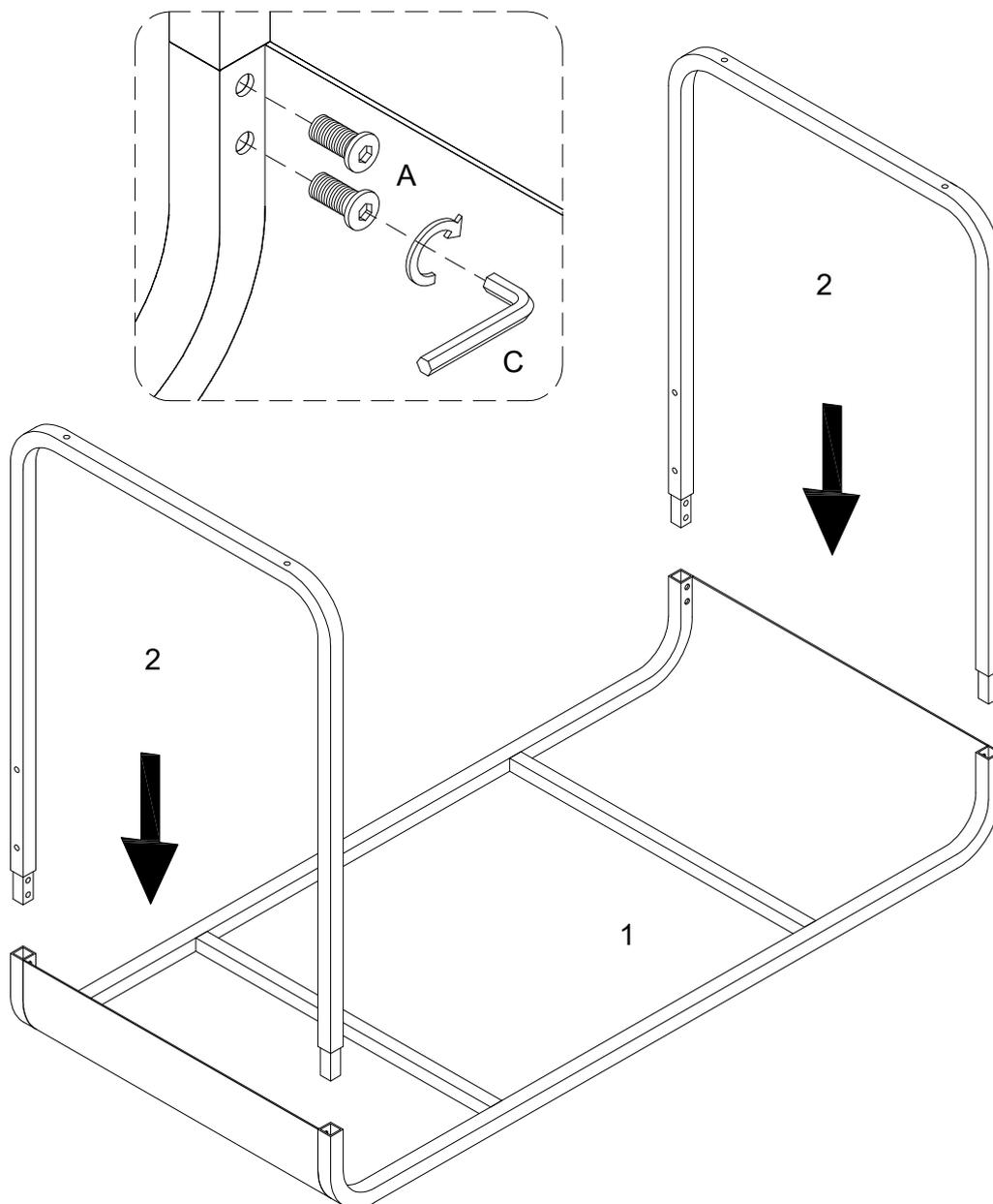
Attach part (2) to part (1) using bolt (A) with hex key (C).
