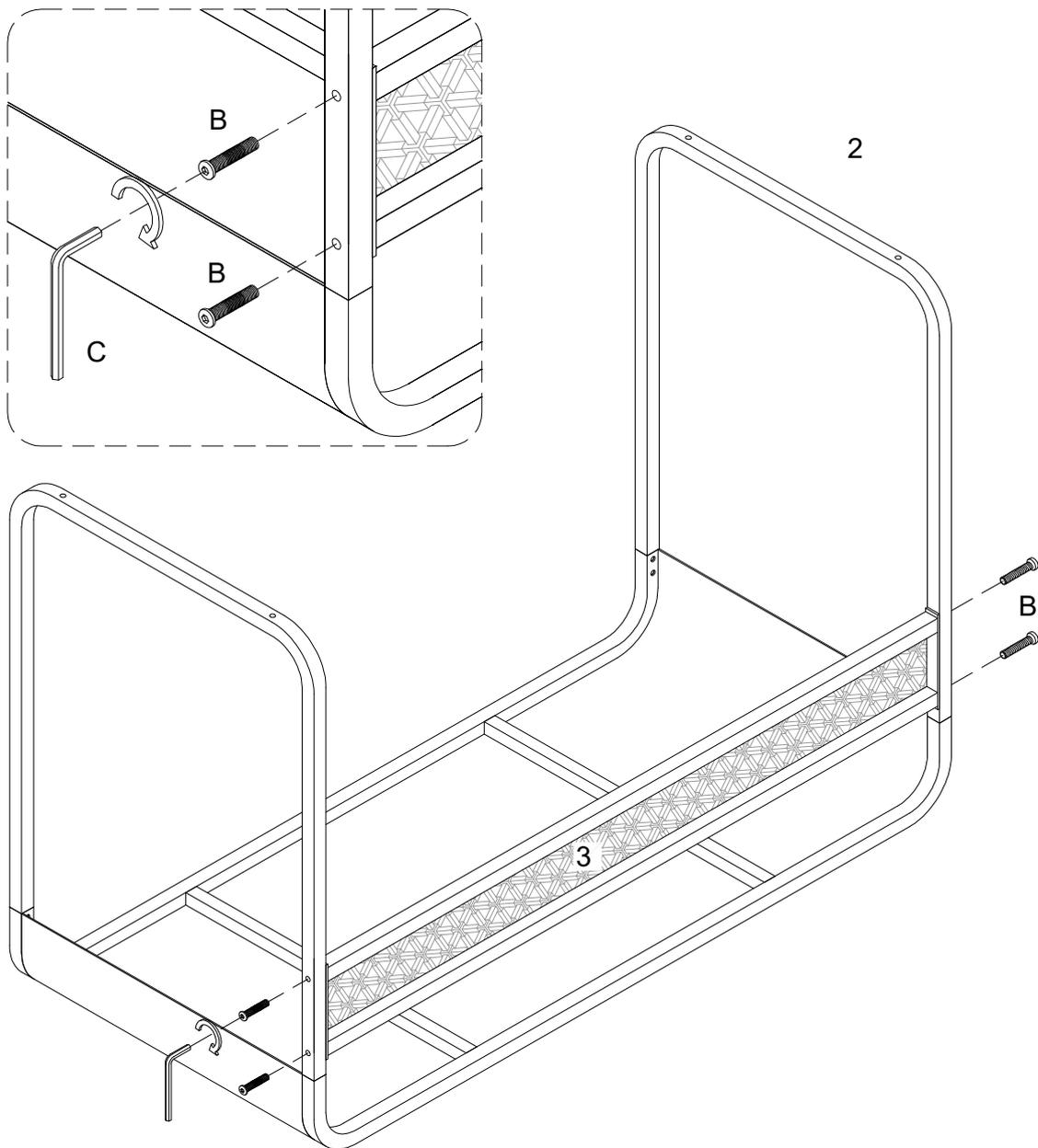
Then using bolt (B) with hex key (C) to secure part (3) to part (2).
