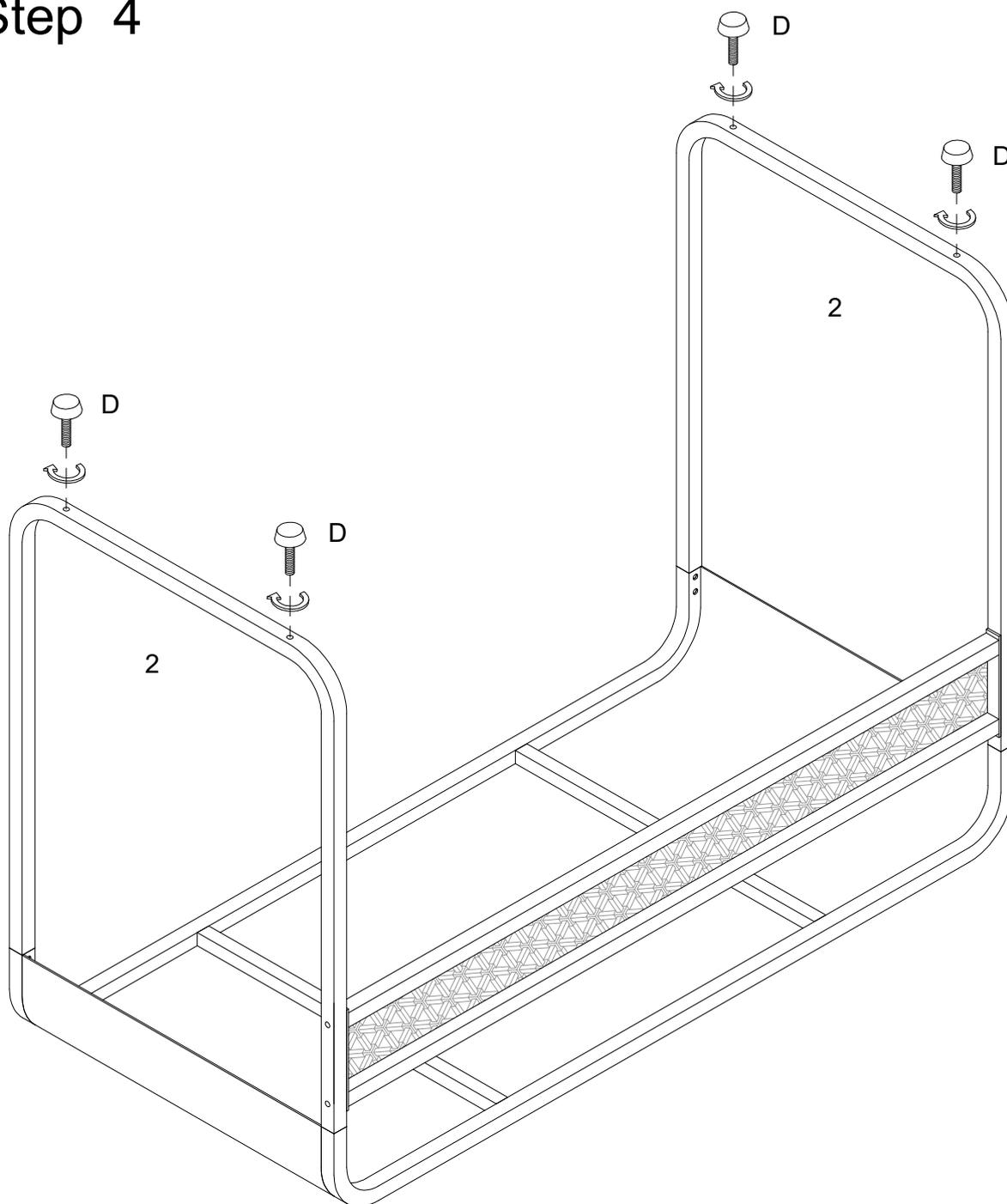
Screw adjustable feet (D) onto part (2) as per diagram.
