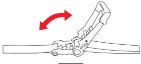
6. Ratchet teeth can damage the line. Keep the line and ratchet straight while cranking and do not over fill the ratchet with the line.
