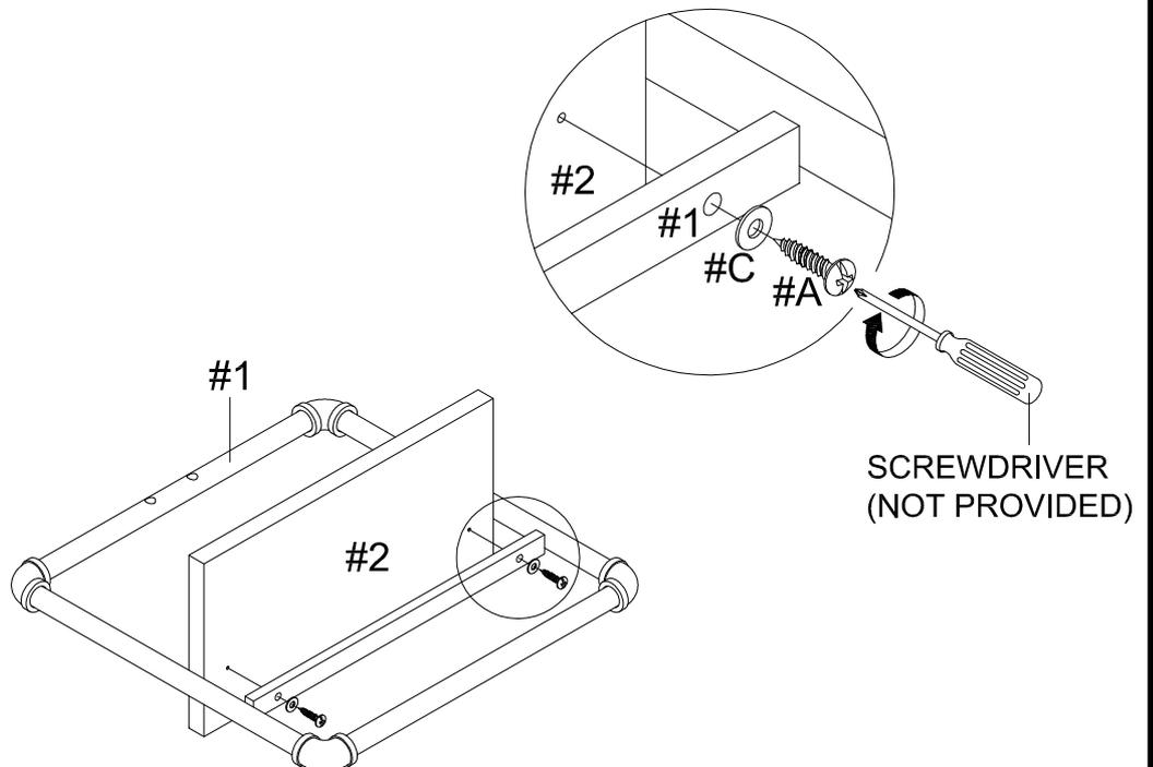
Align shelf (#2) to frame (#1), then secure by using screws (#A) with washers (#C).
