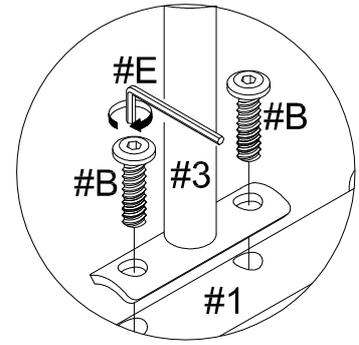
Align supporters (#3) to the frame (#1), then secure by using bolts (#B).
