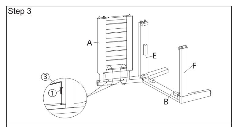
Insert dowels on Backrest Panel(A) into mountings on Left Panel(B). Attach Left Panel(B) to Backrest Panel(A) using Bolts(1) with Allen Key(3). **Do not fully tighten the Bolts.**
