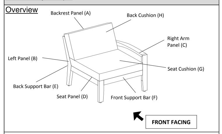
This Right Chair has multiple parts and may require up to 30 minutes to assemble. To give you an overview of the Right Chair parts, the above picture is to help you put the various parts into perspective. Please read through the instructions below to familiarise yourself with the parts and steps before assembly.
