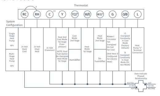
†Internal jumper between RC and RH, located on back of thermostat. †\*Common connection required on Heat-only, Cool-only or Heat Pump systems.
